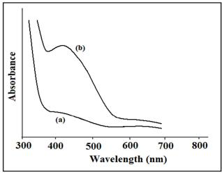
Fig.2. UV-visible absorption spectrum of 0.05% polymer solutions in THF.
