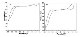
Fig.1. Cyclic Voltammogram of (a) PPAET and (b) PPABT films on ITO coated glass at a scanning rate of 50 mV/S.
