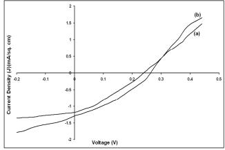
Fig.3. J-V characteristics of photovoltaic devices of the structures (a) (ITO/PEDOT:PSS/PPAET:TiO<sub>2</sub> nanoparticles (1:2 w/w)/ Al) and (b) (ITO/PEDOT:PSS/PPABT: TiO<sub>2</sub> nanoparticles (1:2 w/w)/ Al)
